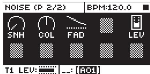
**S&H** (Sample & Hold) sets the tuning of the noise spectrum.
