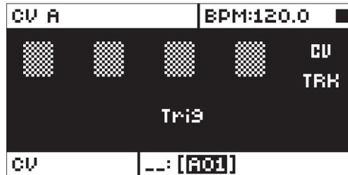
**SRC** (Source Track) sets the track to use for sending trig signals. The CV track, FX track and synth tracks 1-4 can be used as a source.
