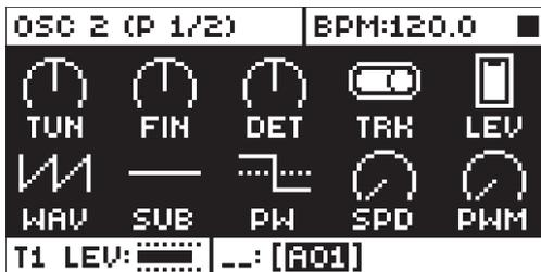
**TUN** (OSC2 Coarse Tune) sets the pitch of the oscillator in semitones. Press and hold **[FUNC]** and then turn the knob to jump a whole octave.
