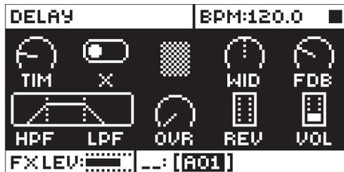
**OVR** (Overdrive) sets how much the delay signal will be overdriven. Please note that higher settings will affect the feedback of the delay.
