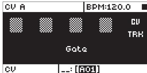
**SRC** (Source Track) sets the track to use for sending gate signals. The CV track, FX track and synth tracks 1-4 can be used as a source.
