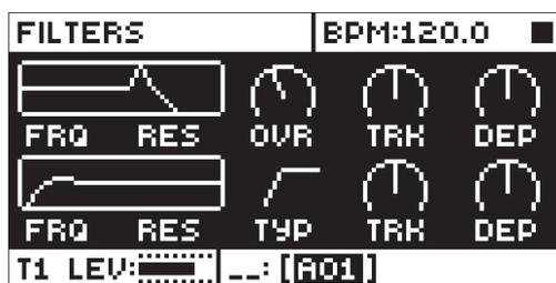
**FRQ** (Filter1 Frequency) sets the cutoff frequency of Filter 1, the 4-pole lowpass transistor ladder filter.
