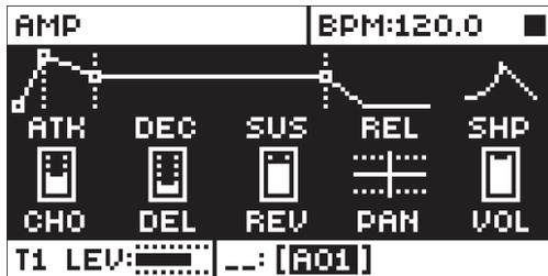
**ATK** (EnvA Attack) sets the attack time of the EnvA envelope, which controls the amplitude of the track.
