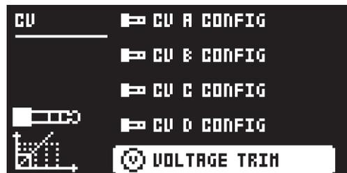
Make sure you have a good voltmeter before proceeding. Connect a TRS cable to the output you want to trim. Connect the voltmeter's negative terminal to the sleeve of the connector. Connect the positive terminal to the tip of the connector.
