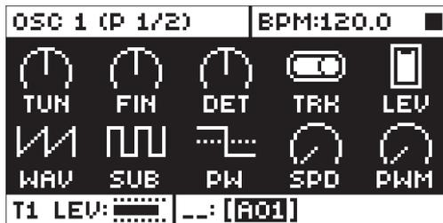
**TUN** (OSC1 Coarse Tune) sets the pitch of the oscillator in semi-tones. Press and hold **[FUNC]** and then turn the knob to jump a whole octave. Press the knob while turning it to jump four semitones.
