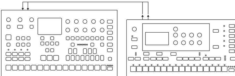
Thanks to the neighbor routing, all the filters of the Analog Four MKII can be used for providing an immense mono filter bank consisting of 8 filters plus 4 overdrive circuits. The setup can be either serial or parallel. It can, of course, be set up for stereo filtering as well. In this scenario, 4 filters are available for the left and right channels.
