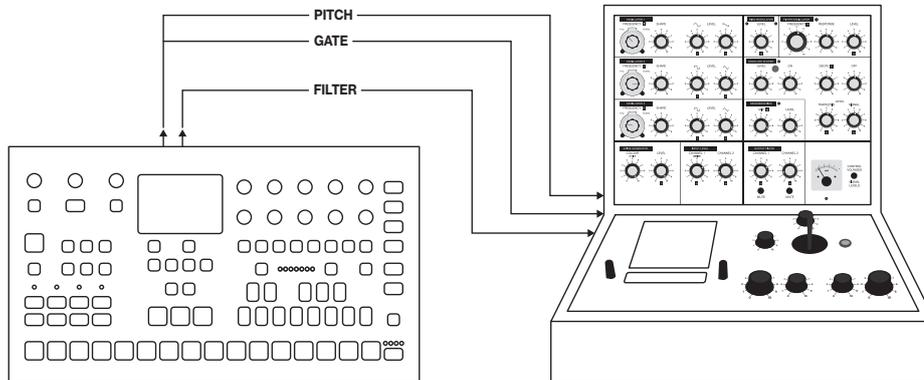
The CV/Gate track of the Analog Four MKII is made for controlling external, CV/Gate equipped, analog gear. In this scenario, a vintage analog synthesizer is controlled by the Analog Four MKII. The pitch and filter cutoff will be controlled.
