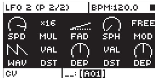
**SPD** (LFO2 Speed) sets the speed of LFO2. It is synced to the BPM. To sync it to straight beats, try settings of 16, 32 or 64. The value is bi-polar (negative values plays the LFO shape backwards).
