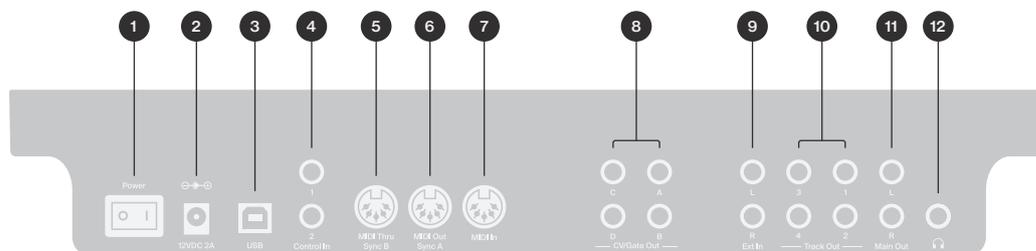
1. **POWER**, For turning the unit on and off.
