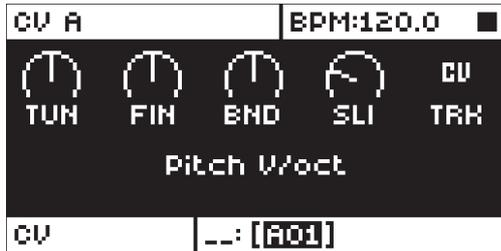
**TUN** (Coarse Tune) sets the coarse tuning of the CV in semitones.
