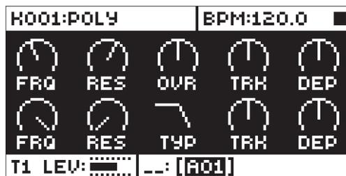
6. Place note trigs on the first step of the sequencer. Triggering the amplitude envelope is necessary.
