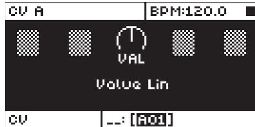
**VAL** (Value) sets the voltage level of the CV. Applicable when the chosen CV type is VALUE LIN.
