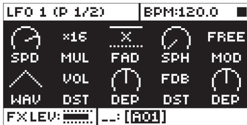
**SPD** (LFO1 Speed) sets the speed of LFO1. It is synced to the BPM. To sync it to straight beats, try settings of 16, 32 or 64. The value is bi-polar (negative values plays the LFO shape backwards).
