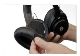
To replace the earpad, place it onto the earcup and start to slowly work the outer edge of the earpad into the groove.
