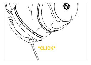
→ To remove or replace the cable, pull it gently out of the connector using the barrel of the jack connector, not the cable.
