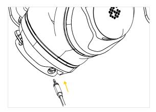
→ Insert the connection cable into one of the connectors until it locks into place with an audible click.
