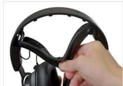
To replace the headband padding, insert one end into the end cap then clip the padding on the headband, starting from the inserted end and working towards the other. Insert the far end into the other end cap. You may need to open the headband wide to finish installing.
