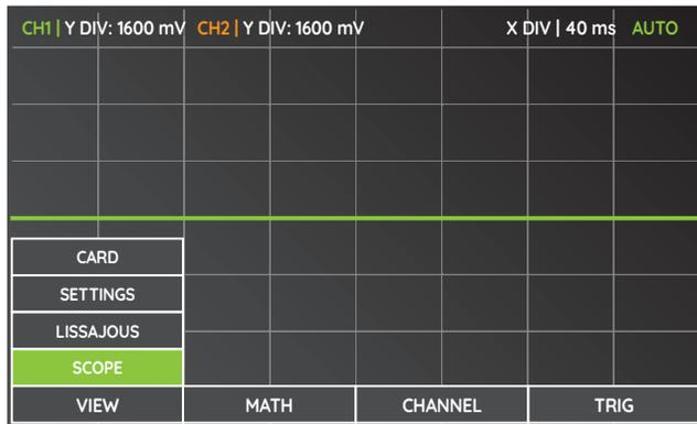
As you flip the MENU switch, the configuration menu appears. In the first submenu, you can set the basic functions of the unit. The options (from bottom to top) are: OSCILLOSCOPE, LISSAJOUS FIGURES, MASTER SETTINGS AND CONFIGURATION, VOICE CARD CONFIGURATION. Rotate the Y encoder to select the relevant feature and push the Y encoder to confirm.
