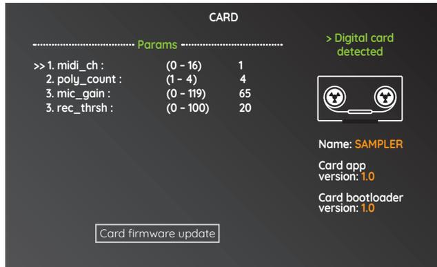
The CARD screen is available only if a digital voice card (Sampler/Looper, Gesture controller) is inserted in the voice card slot.
