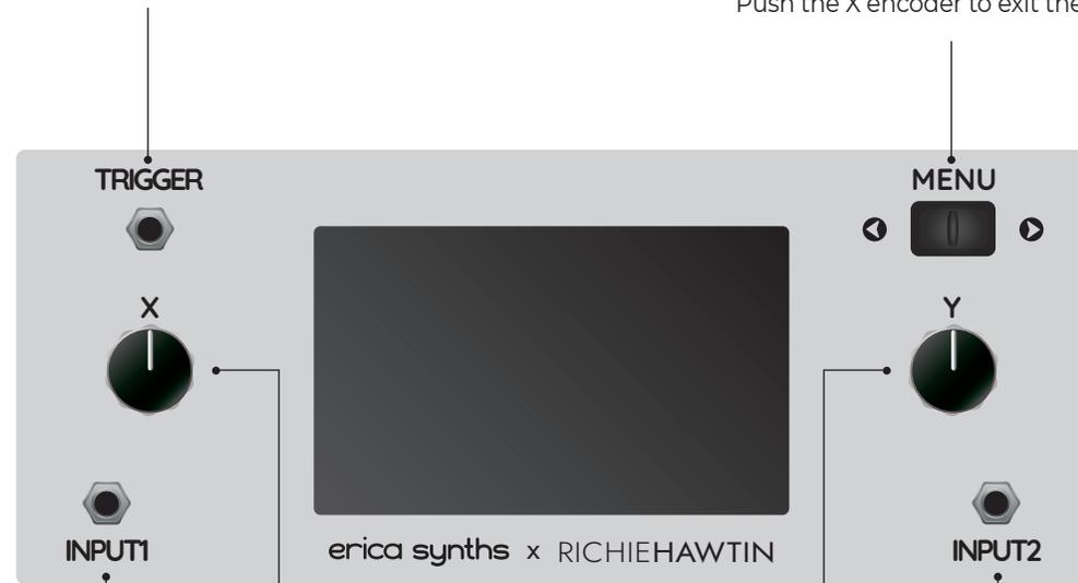
This is the input of the first (green) channel of the oscilloscope.
