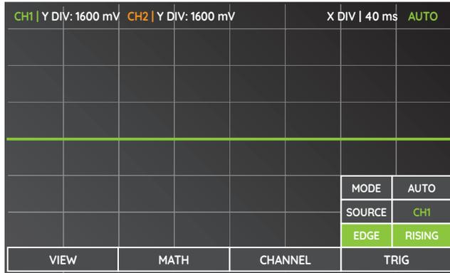
In the TRIG menu you can configure the oscilloscope trigger settings – a moment of time (or you can imagine it as a point on the X axis on the oscilloscope screen) at which the waveform drawing is refreshed. This allows for a nice, static representation of the waveforms on the oscilloscope screen.
