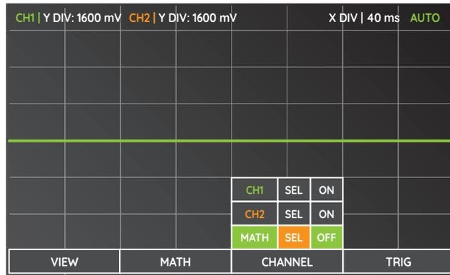
In the CHANNEL menu, you can activate and deactivate the oscilloscope channels. There are two channels available, represented by INPUT 1 and INPUT 2 and one virtual channel – MATH, that visualizes the sum or multiplication of the incoming signals. Each channel has two settings – SEL (select) and ON/OFF.
