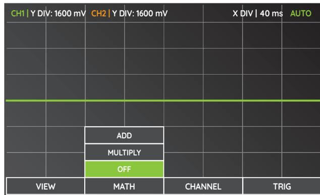
In the MATH menu you can ADD or MULTIPLY signals applied to channels 1 and 2 of the oscilloscope. The resulting waveform is represented by a yellow color. This feature is very useful to illustrate and visualize different new waveform synthesis techniques.
