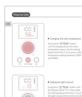
• Setting the light channel Long press "CCT|CH" button until the display shows "CH", then rotate the Setting Adjustment Dial ① to set
