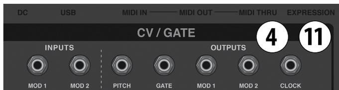
These seven connectors allow the Hydrasynth to interface with the wild and wonderful world of modular synthesizers. There are five outputs (Pitch, Gate, Mod 1, Mod 2, and Clock) and two
