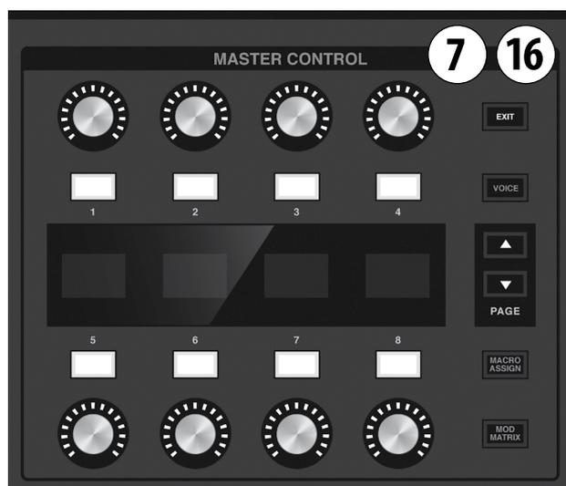
If you like to make your own patches, you might enjoy this top-panel section the most. When a Module is accessed the parameter values are shown in the Right display, selected with the Control buttons, and adjusted with the Control knobs. The Page Up/Down buttons provide access to more parameters whenever a Module offers more than eight. We'll cover the parameters of each Module in [Hydrasynth Desktop \(p. 24\)](#).
