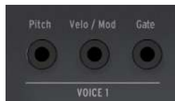
CV Gate outputs
