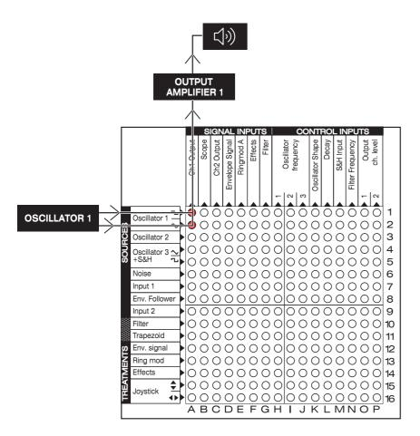
In this basic patch both pulse and sine output signals from the Oscillator 1 go directly into the input of the Output amplifier of the Channel 1. Make Channel 1 level is set at desired value and Panning is at middle. Nothing interesting here, but we have a sound on the output. By adjusting Frequency dial on the Oscillator 1 you can alter the pitch of the sound and by adjusting waveshape and level controls, you can alter the timbre of the sound.
