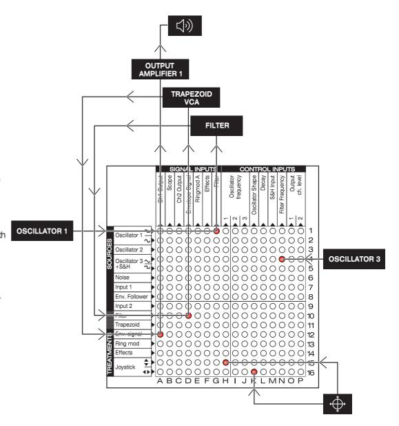
This is an example of the patch that provides stereo panning effect. The pulse wave signal from the Oscillator 1 goes to both Output Channel 1 and Output Channel 2. Make sure, both LEVEL knobs on the Output Amplifiers are set to desired volume and the Channel 1 is panned all way left, while the Channel 2 is panned all way right.
