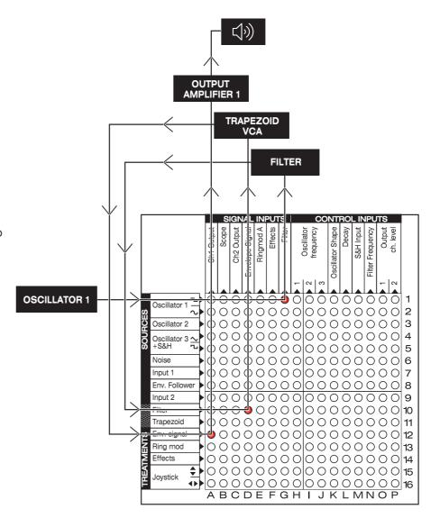
In this patch the pulse wave signal from the Oscillator 1 goes into the input of the Filter and the output of the Filter is patched into the VCA (Envelope signal) linked to the envelope generator (Trapezoid). The signal form the VCA output goes into the Output amplifier of the Channel 1.
