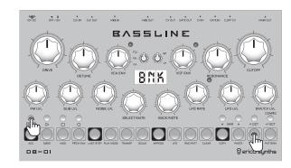
The Bassline DB-01 has a memory of 8 banks of 16 patterns. Before you start designing a pattern, you must select the bank that you need for pattern saving/loading. To do so, push and hold the SHIFT button and push the BANK button. The first ten step buttons will appear 70% dimmed, representing the available banks, and the banks with some patterns saved already will appear fully lit. Just push one of the bank buttons to select a bank. To return to the step enter menu, push the BACK/NOTE encoder.
