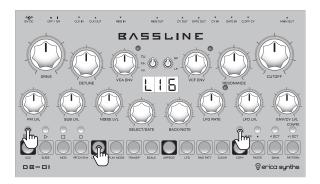
Push and hold the SHIFT button and push the LAST STEP button! Now you can rotate the NOTE encoder or push one of the step buttons to set the last step. For sequences longer than 16 steps use the BAR buttons to access the bars of 16 steps, and push the step button to set the last step. The indicator will show the last step of the sequence. You can also set the play-head to follow the bars automatically. See the configuration settings in this manual!
