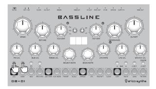
You can play the Bassline DB-01 like a regular keyboard without a sequencer running. To do so, stop the sequencer, push and hold the SHIFT button and push the PLAY button. The step buttons will light up 50% and 70% dimmed, emulating the piano keyboard. Now you can simply play the keyboard and use the -10CT and +10CT buttons to transpose the keyboard. Take note that the keyboards change according to the set scale on the scale menu. Rotate the SELECT/GATE encoder to set master glide amount.
