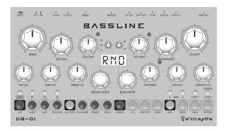
In order to have nice unpredictability when working with DB-01, the pattern randomization is implemented. You can randomize all pattern settings or specific parts (notes, gates, accent, slide, modulation track, etc.) of it. To start pattern randomization, push and hold the SHIFT button and push RND PATT button! The sequencer now is in randomization mode, and parameters available for randomization are lit on the step buttons.
