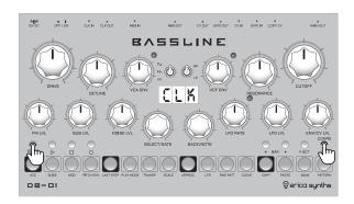
In the configuration menu, you can configure different parameters for the Bassline DB-01. To access all the configuration functions below, push and hold the SHIFT button and push the CONFIG (+1 OCT) button!
