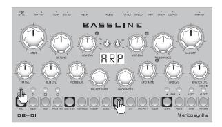
The DB-O1 has a built-in arpeggiator. It can work in two ways – it can create simple arpeggios or insert arpeggios into the sequence.
