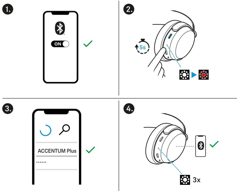
**i** If no connection is established within 2 minutes, pairing mode is terminated and the headphones switch to standby mode. If necessary, repeat the steps described above.
