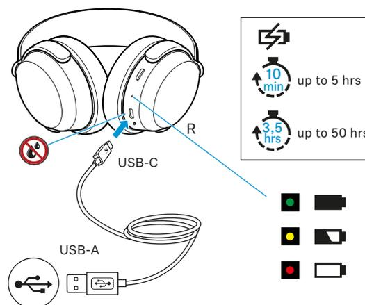
1. Make sure that the charging socket is free from moisture and contamination. Connect the USB-C connector of the charging cable to the USB socket of the headphones.
