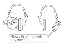
In order to support a wide variety of monitoring styles, this product has been designed with the ability to swivel the ear pieces front-to-back, and rotate each earpiece housing to the outside. Before using, however, please confirm the correct direction and degree of movement allowed, and do not apply excessive force in the attempt to swivel, rotate, or bend the headphones in ways not supported, since damage may result.
