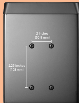
Fig. 2: Bottom of the SM-5 showing mounting hole position and spacing.
