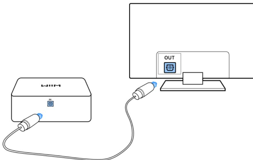
**Note:** The **Optical In** interface on the WiiM Vibelink Amp supports **PCM** audio format only. Please ensure that the audio source device connected to the WiiM Vibelink Amp is set to output audio in **PCM** format. Otherwise, you may not hear sound.
