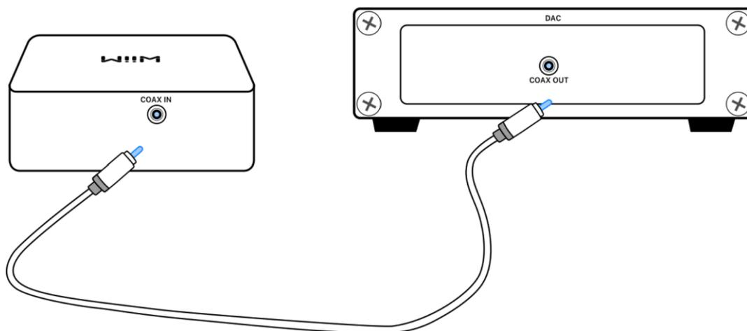
**Note:** The **COAX In** interface on the WiiM Vibelink Amp supports **PCM** audio format only. Please ensure that the audio source device connected to the WiiM Vibelink Amp is set to output audio in **PCM** format. Otherwise, you may not hear sound.
