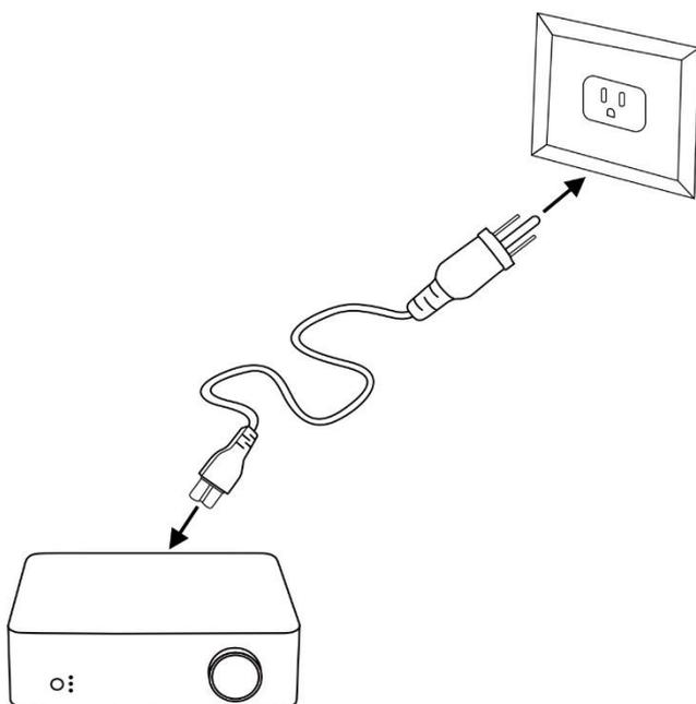
Use the supplied AC power cable to connect the WiiM Vibelink Amp to a power outlet. This cable is specifically designed to support a wide range of voltages, accommodating 100-240V AC, 50/60 Hz with a maximum current of 3A. This flexibility ensures that the WiiM Vibelink Amp can be safely and effectively powered in various locations.
