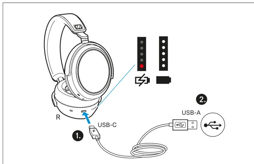
1. Connect the USB-C connector of the charging cable to the USB socket of the headphones.
