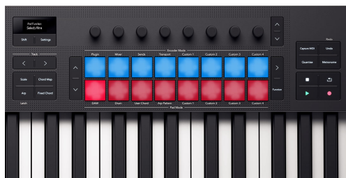
The Launchkey's pads in Logic's Select/Arm mode.
