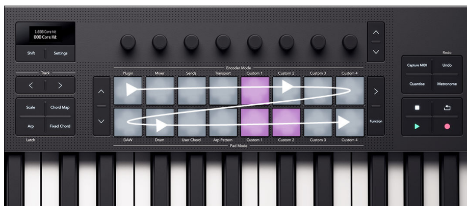
Pad layout with arrows showing the direction of the sequencer
